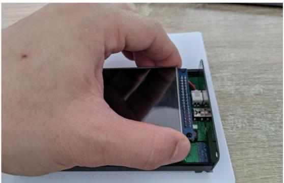
For a new device, the battery must be purchased separately - battery parameters are given in point 1. For the device after repair, use the old battery, but check for damage before installation. Peel off the protective layer on the adhesive tape, glue the battery evenly and assemble the device in the reverse order (connect the battery, install the screen, screw the top cover).
