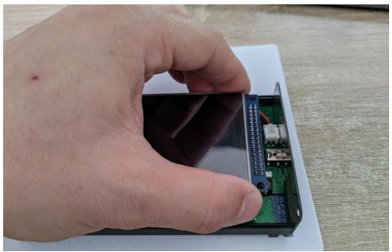
The battery is held on with adhesive tape. It can be removed by taking a flexible thin plastic plate (like a bank card) and moving it, placing the short side between the middle of the battery and the board.
