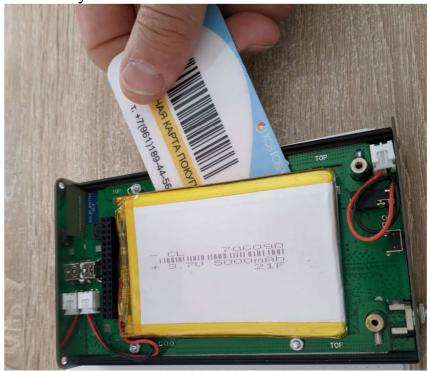
Disconnect the power connector by pulling it out of the mating connector on the board.
