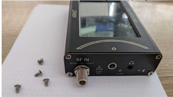
Unscrew the 2 shield fixing screws and hold the shield board on the solder pin side (opposite the round mounting holes), rock it outward and disconnect.
