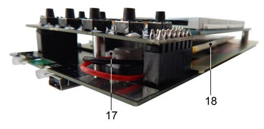
Figure 9.4.3 – Replacing the battery
