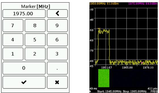
Figure 8.6.2 – Entering the marker frequency and displaying the markers on the screen
