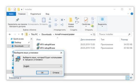
Figure A1.4 - Select the language to be used during the update loader installation
