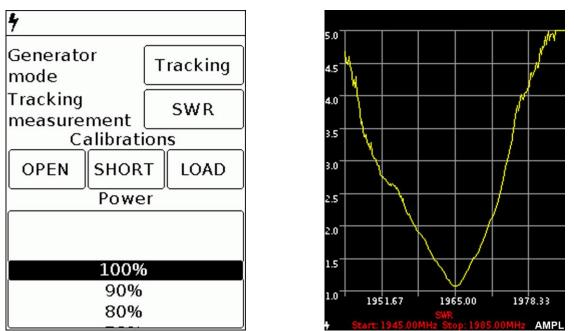
Figure 8.4.6 - Measurement the standing wave ratio in the SWR mode
