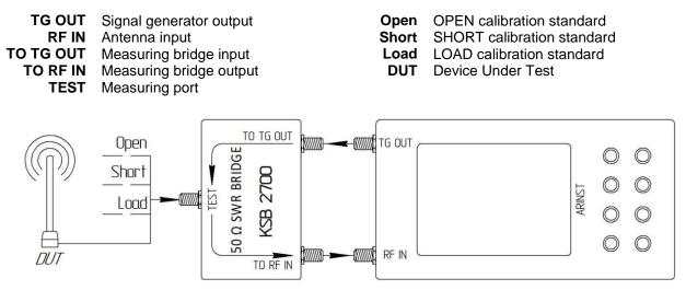
Figure 8.4.5 – Connecting the measuring bridge to the spectrum analyzer
