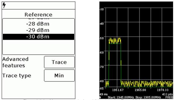
Figure 8.5.3 - Measurements in the additional mode «Trace Minimum»
