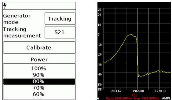
Figure 8.4.3 – Measurement of the amplitude-frequency characteristics of the equipment under test
