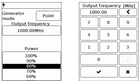
Рисунок 8.4.2 – Setting the frequency and power of the signal in the «Point» mode
