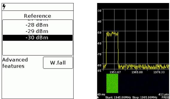
Figure 8.5.5 - Measurement in the «Waterfall» mode
