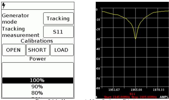
Figure 8.4.4 - Measurement of the reflection coefficient
