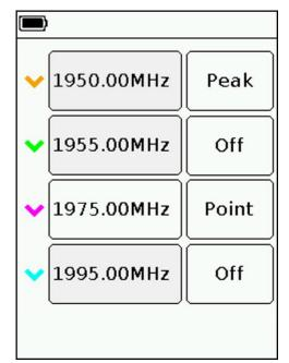
Figure 8.6.1 – Menu for setting markers and displaying peak values
