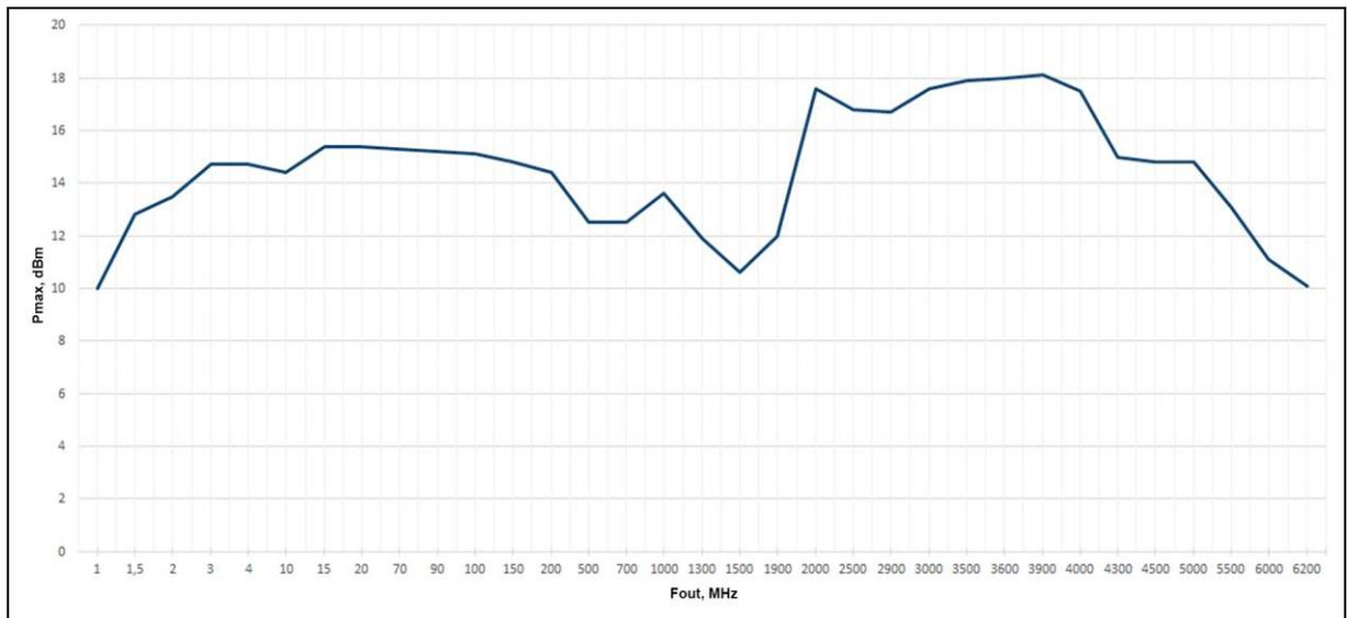
Figure 3.1 – Maximum output power level of the ARINST ArSiG-S generator
