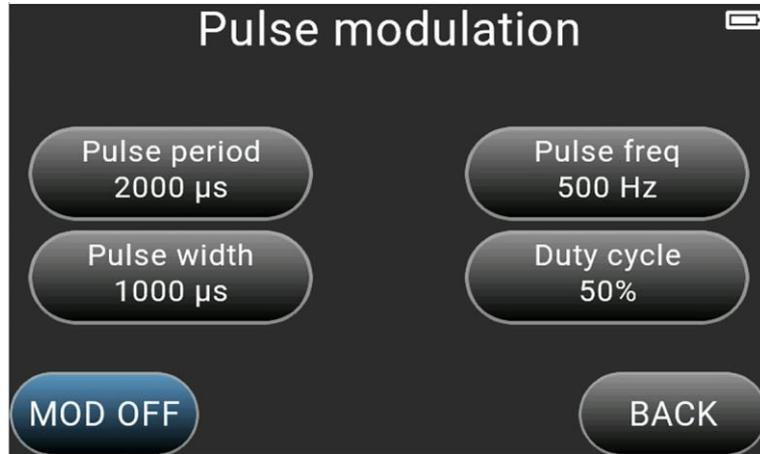
Figure 10.2 – Pulse modulation menu
