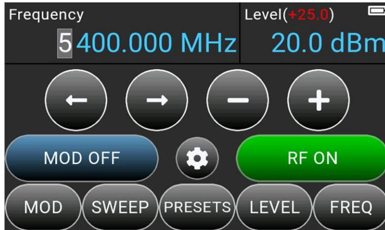
Figure 10.10 – Signal power level offset enabled
