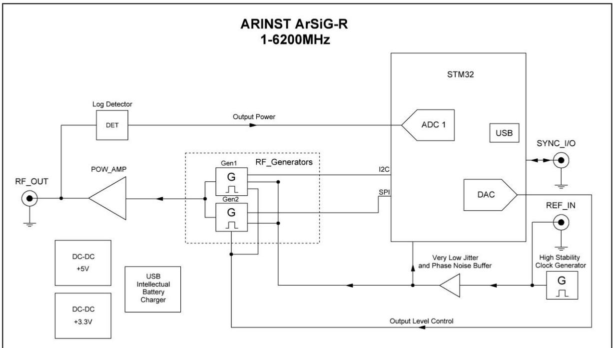
Figure 6.2 - Block diagram of the ARINST ArSiG-R signal generator
