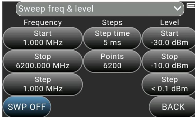
Figure 10.4 – Signal output menu in sweep mode
