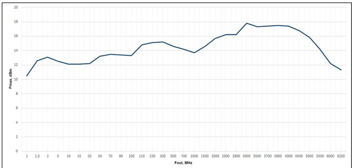
Figure 3.2 – Maximum output power level of the ARINST ArSiG-R generator
