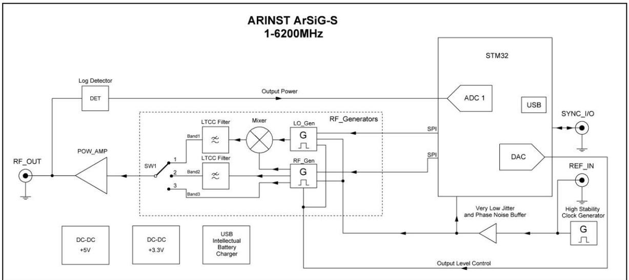
Figure 6.1 - Block diagram of the ARINST ArSiG-S signal generator
